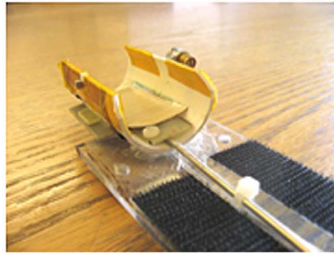
Figure 1. RF coil used for image acquisition. The dual frequency coil combines a Helmholtz pair proton coil (transmit and receive, 200 MHz) nested on a single loop ^{129}\text{Xe} coil (transmit and receive, 55.35 MHz). This coil architecture allowed proton and ^{129}\text{Xe} images to be acquired sequentially while maintaining exact co-registration (Clinical MR Solutions, Brookfield, WI). The two coils were intrinsically decoupled.
